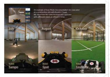
Automated Approach: Faster and simpler automated 360° photo documentation for construction projects, replacing manual methods.
